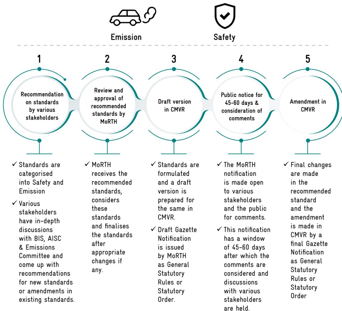
Figure 8 - Flow chart for amendments to technical standards for emission and safety
